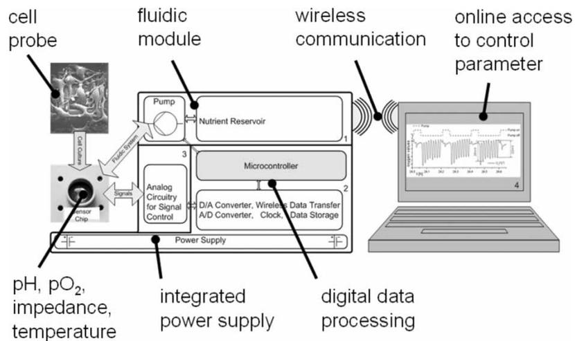
**Figure 4.** Modular set up of the IMOLA system: 1) fluidic module, 2) analog module including sensor chip with cell probe, 3) digital module including wireless communication and data processing, 4) software module. Furthermore an integrated power supply is included.
