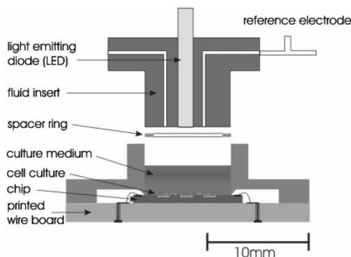
**Figure 2.** Cross section of the biosensor chip and live support system which was developed at the Heinz Nixdorf-Department for Medical Electronics.
