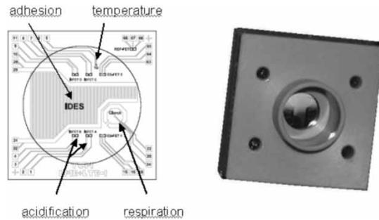
**Figure 5.** Layout (left) and encapsulated silicon biosensor chip (right) (produced by Heinz Nixdorf-Department of Medical Electronics). An amperometric sensor is used for measurement of  $pO_2$ , for impedance measurement an IDES sensor is used. pH measurement is performed by ion sensitive field effect transistors (ISFET). Side length of one chip is 24 mm, the cell culture area has a diameter of 6 mm. A temperature diode is integrated for control purposes.
