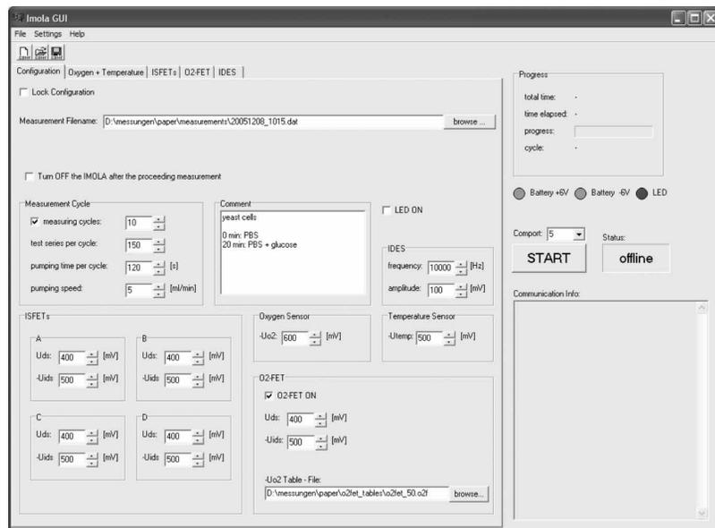
**Figure 8.** Software configuration menu for measurement cycle adjustment and for control of the microsensors.
