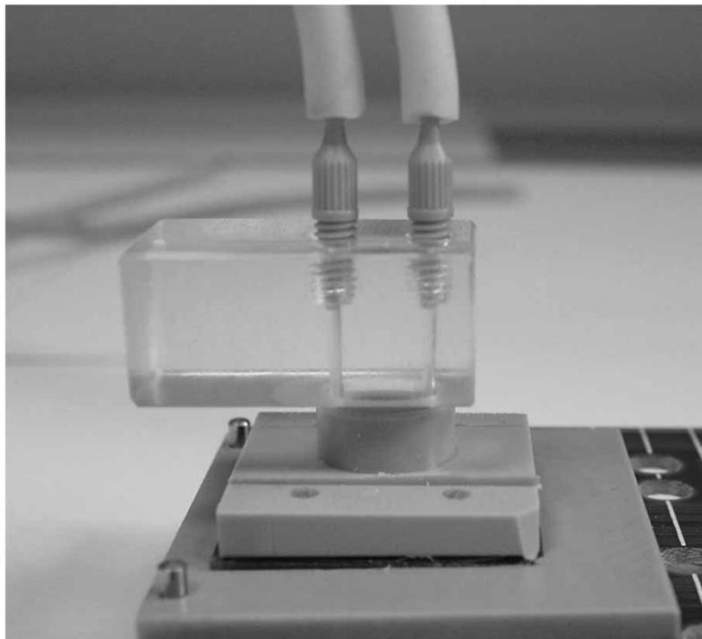
**Figure 1.** Connector, sensor chip, fluid insert, and fluidic connectors. The sensor chip (middle) is set into the connector socket (height 3,0mm) to contact the control PCB electronically. The fluidic adapter is pressed into the round cell culture well and seals it. Inflow and outflow tubes are plugged onto standard fluidic connectors (LED inlet not shown). The transparent fluidic adapter has a mechanical extension for easier handling.
