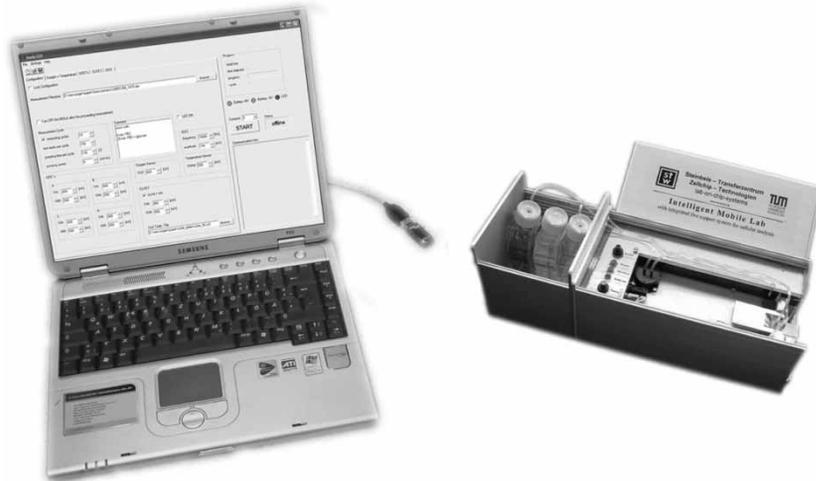
**Figure 3.** Intelligent Mobile Lab device (produced by Steinbeis Transferzentrum-Lab on Chip Systems, Bernreid, Germany). The front part on the right (size: 210 mm × 105 mm × 90 mm) incorporates the analog and digital electronic circuitry, the biosensor and the live-support system. The back part (size: 90 mm × 105 mm × 105 mm) includes the reservoir and waste tanks and provides an external antenna. The software module is shown on the left running at a laptop.
