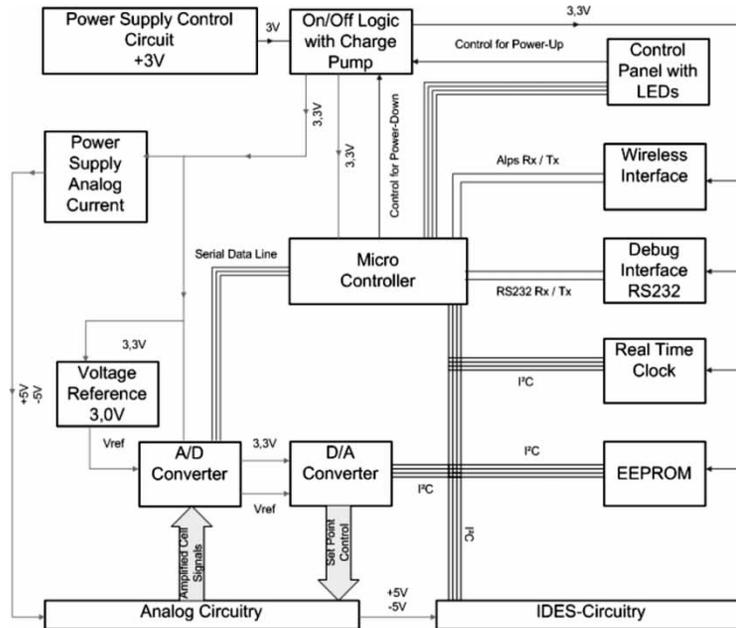
**Figure 7.** Architecture of digital data management module. Core is the PIC 16F777 microcontroller. The control panels are connected to digital outputs. Two RS232 ports are implemented for connection of the wireless interface and for the debug plug. The D/A converter, the buffer, the clock, and the IDES circuitry are connected via an I<sup>2</sup>C—bus (Wiest et al. 2005c). The A/D converters are connected directly via a fast serial bus.
