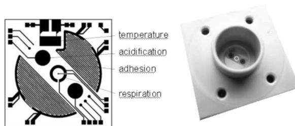
**Figure 6.** Layout (left) and encapsulated ceramic biosensor chip (right) (produced in cooperation by Heinz Nixdorf-Department for Medical Electronics and Herqeus Sensor Technology). An amperometric sensor is used for measurement of  $pO_2$ , for impedance measurement an IDES sensor is used. pH measurement is performed by an metal oxide sensor. Side length of one chip is 24 mm; the cell culture area has a diameter of 6 mm. A Pt1000 is integrated for temperature control purposes.
